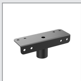
Pole mounting adaptor Q235 steel, cold galvanized, ecoating with powder coating. Code: BC-F08-02(dia.42mm) Code: BC-F08-03(dia.76mm)
